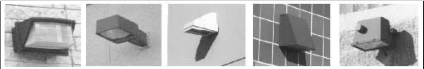
The fixture at far left is commonly referred to as a "wallpack" type. It represents a category of poorly designed luminaires that will perform most lighting tasks badly, casting glare in all unwanted directions. The remaining fixtures shown are all cutoff or equivalent. The fixture at far right is a floodlight installed in a cutoff position. The four fixtures at the right provide excellent lighting without unnecessary light pollution.
